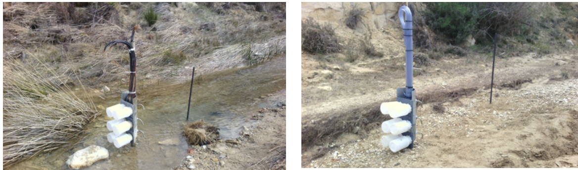
Picture 2.2.10.2 Siphon samplers placed in an intermittent (left) and ephemeral (right) stream in a semi-arid catchment in Murcia (SE Spain). Multiple samplers are spaced vertically to collect suspended-sediments samples at different depths during a flooding event. Photo: María Almagro.
