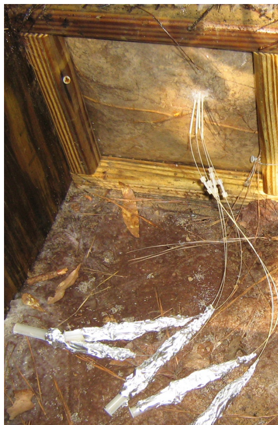
Figure 2.1.5.2 Micro-suction cups installed in a rhizobox (photo credit: Ina C. Meier).
