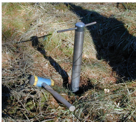
Picture 2.1.2.1 Root sampling with the soil coring method in forests. The O-horizon is first sampled within the wooden frame (25 x 25 cm) down to the top of the mineral soil and the height of the O-horizon is measured at least at 5 positions along the edge of the frame. Next, soil and roots are sampled, (here from 0-30 cm with a 5 cm diameter auger). The same soil pit can be used for installation of root ingrowth cores. (Photo: Inger Kappel Schmidt)
