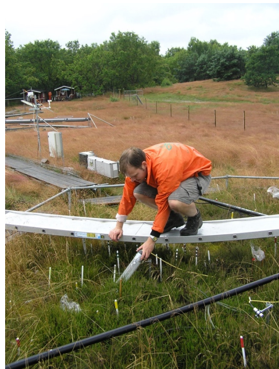
Photo 2.1.2.2 Installation of a mini-rhizotron. (Photo: Inger Kappel Schmidt)
