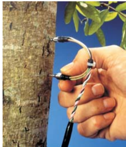
Figure 3.7.3 A thermal dissipation sensor as manufactured by Dynamax .
