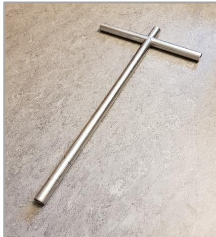
**Figure 4.10.2** Metal soil corer used for mesofauna samples (left; photo: Heidi S. Konestabo) and a tubular soil probe commonly used to collect soil samples for nematode extraction (right; photo: Paul Kardol).
