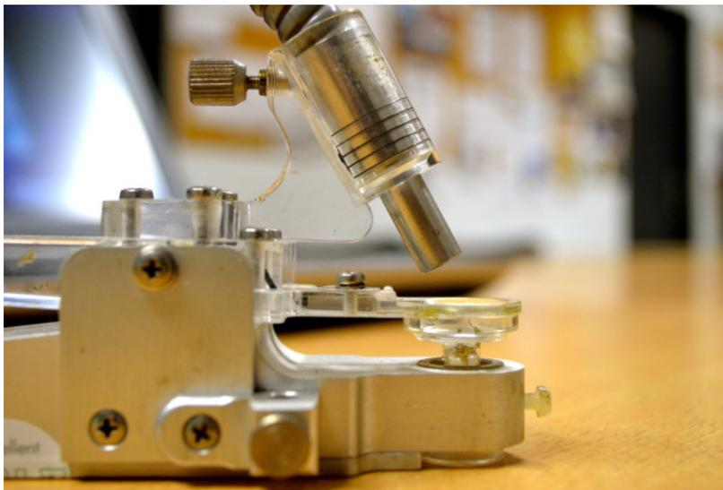
**Figure 5.1.3** Leaf clip of a pulse amplitude modulated (PAM) fluorometer, with different light sources from above and below. A leaf – potentially still attached to the plant – is held underneath the horizontal plate. Photo: Jonas Lambrechts.
