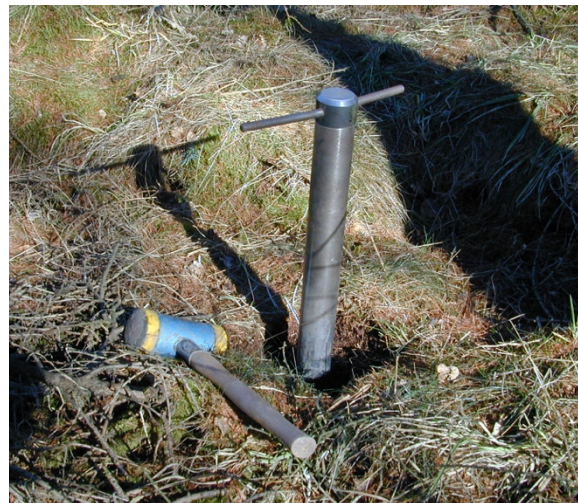
Picture 2.1.2.1 Root sampling with the soil coring method in forests. The O-horizon is first sampled within the wooden frame (25 x 25 cm) down to the top of the mineral soil and the height of the O-horizon is measured at least at 5 positions along the edge of the frame. Next, soil and roots are sampled, (here from 0-30 cm with a 5 cm diameter auger). The same soil pit can be used for installation of root ingrowth cores. (Photo: Inger Kappel Schmidt)
