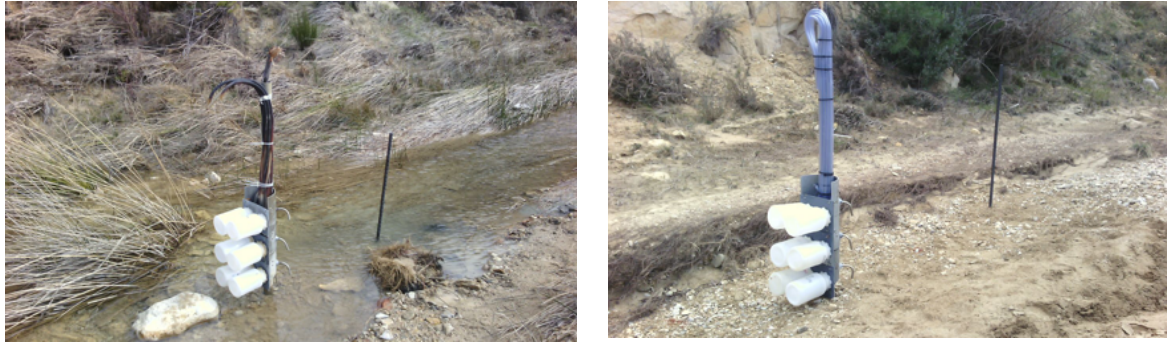
Picture 2.2.10.2 Siphon samplers placed in an intermittent (left) and ephemeral (right) stream in a semi-arid catchment in Murcia (SE Spain). Multiple samplers are spaced vertically to collect suspended-sediments samples at different depths during a flooding event. Photo: María Almagro.
