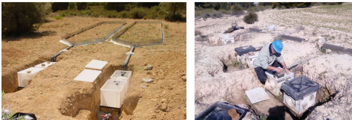
Picture 2.2.10.1 Bounded (left) and unbounded Gerlach-type (right) erosion plots connected to sediments and runoff collecting tanks in two study sites in Murcia (SE Spain). Photo: María Martínez-Mena (left) and Eloisa García (right)
