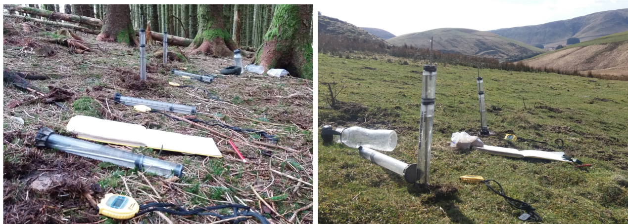
Figure 3.2.1 Setup of infiltration measurements in a forest (left) and on a grassland soil (right) using mini-disk infiltrimeters and stop watches. Photo: Francis Parry (Centre for Ecology & Hydrology).
