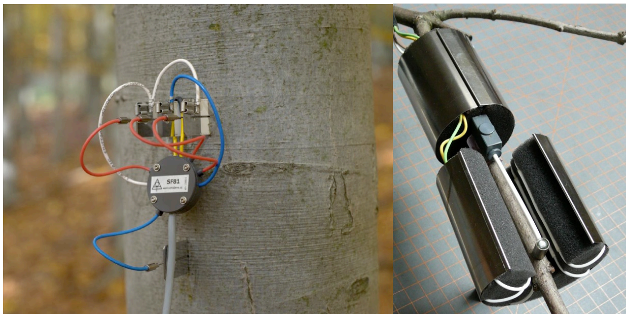
Figure 3.7.1 THB sap flux sensor (left) and “baby” THB sensor manufactured by EMS (right).
