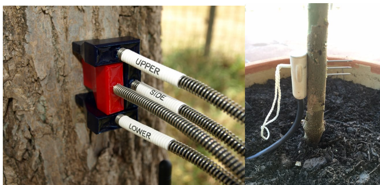
Figure 3.7.2 HFD sensor HFD8-100 manufactured by ICT international (left) and HPV sensor manufactured by Edaphic Scientific (right).
