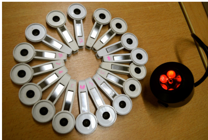
Figure 5.1.2 Dark adaption clips and optical sensor unit (with measurement light) of a plant efficiency analyser (PEA). The dark adaption clip is installed on a leaf and the metal shutter is used to close the measurement hole. After dark adaption time of 15-20 minutes, the sensor unit is placed on the clip, the shutter is opened and the measurement light flashed. Photo Jonas Lambrechts.
