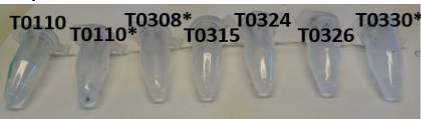
Figure 4: Activity of enzymes with indole as substrate. Indole is turned in the reaction into indigo, which is blue. The reaction had an enzyme concentration on 100 nM and an indole concentration on 2.4 mM. The enzymes marked with * had NADPH as co-factor, while the rest had NADH. The image was taken approx. 25 hours after start of reaction, and the samples had been centrifuged.
