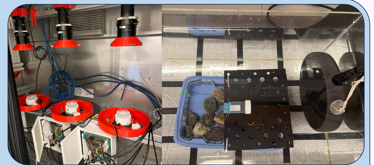
Figure 1. Noise exposure stations. 110dB control. Left: Tracking station containing speaker. Right: Calibrated tank with underwater speaker.
